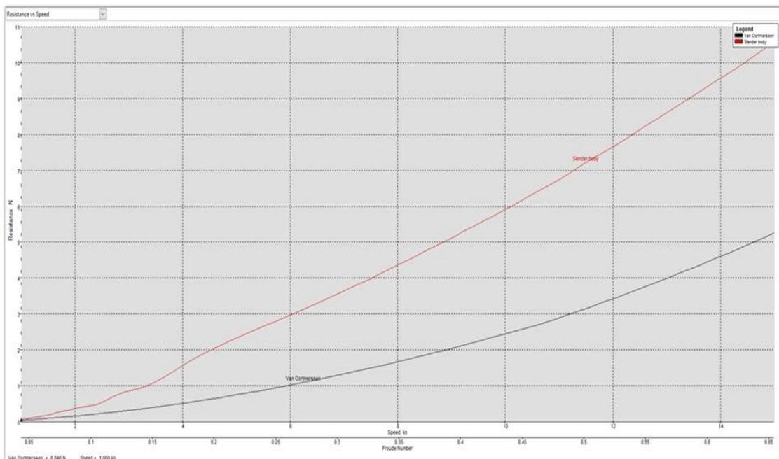
Figure 8: Resistance vs Speed Graph (Waterjet) is made by Maxsurf Resistance
