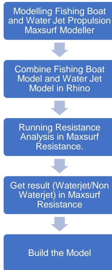
Figure 1: Simplified diagram of the flow chart
