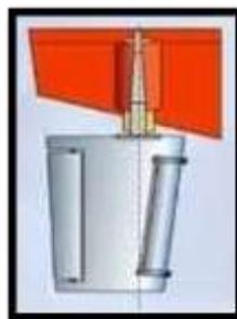
Figure 3: Design Combined Flap, Rotor Rudder (T- Rudder)
