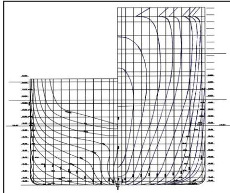
Figure 3: MTL036B Body Plan
