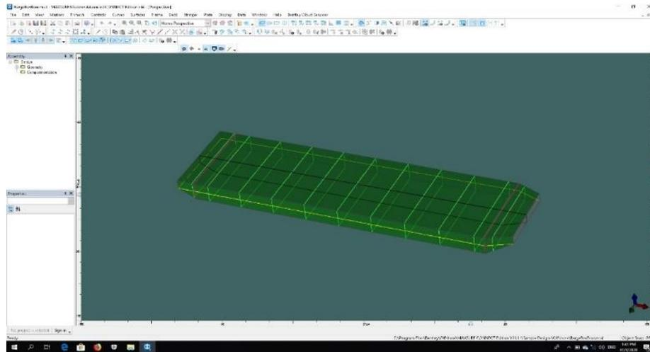
Figure 8: Hull modelling in MAXSURF Modeler
