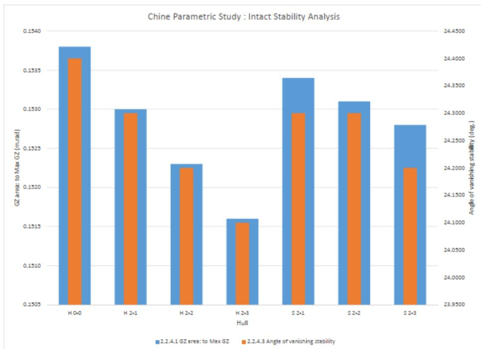
Figure B: Comparison of Chine with Same Chine Width of 2 feet
