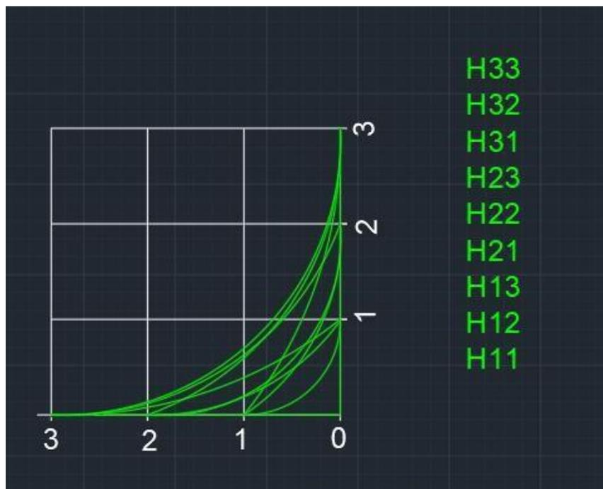
Figure 6: Example parametric study for soft chine shape
