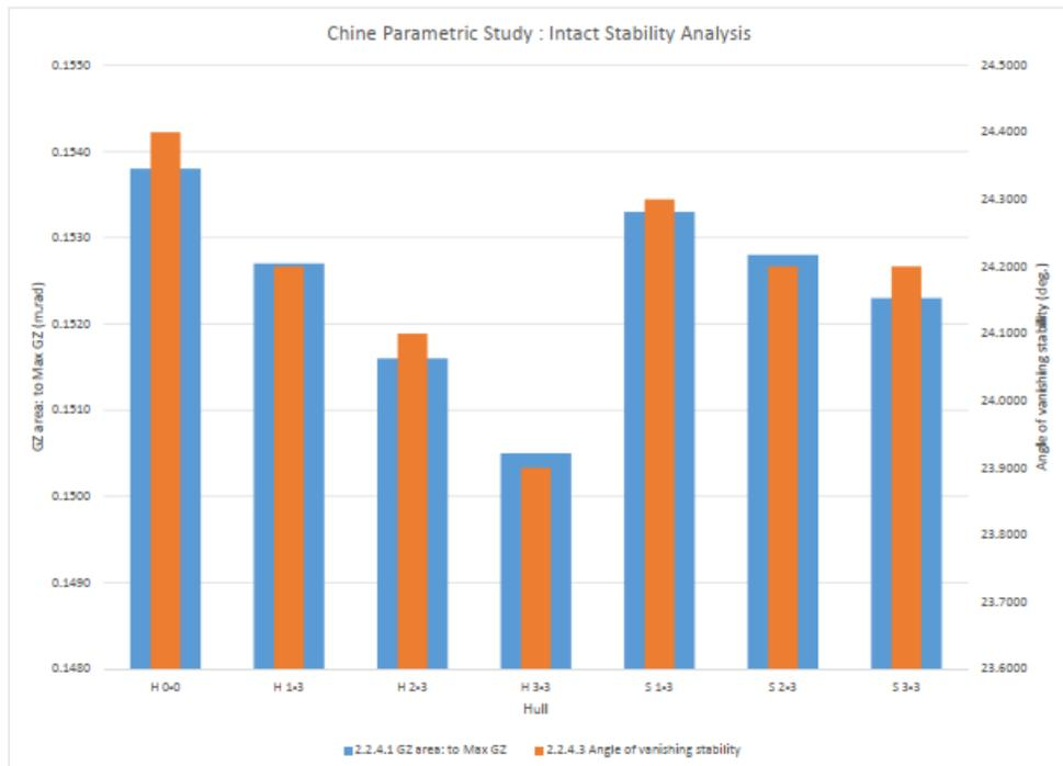
Figure D: Comparison of Chine with Same Chine Height of 3 feet
