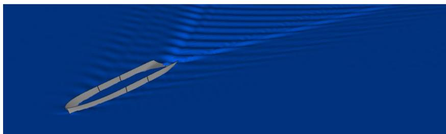
Figure 7: Wave pattern Fishing Boat at 15 knots
