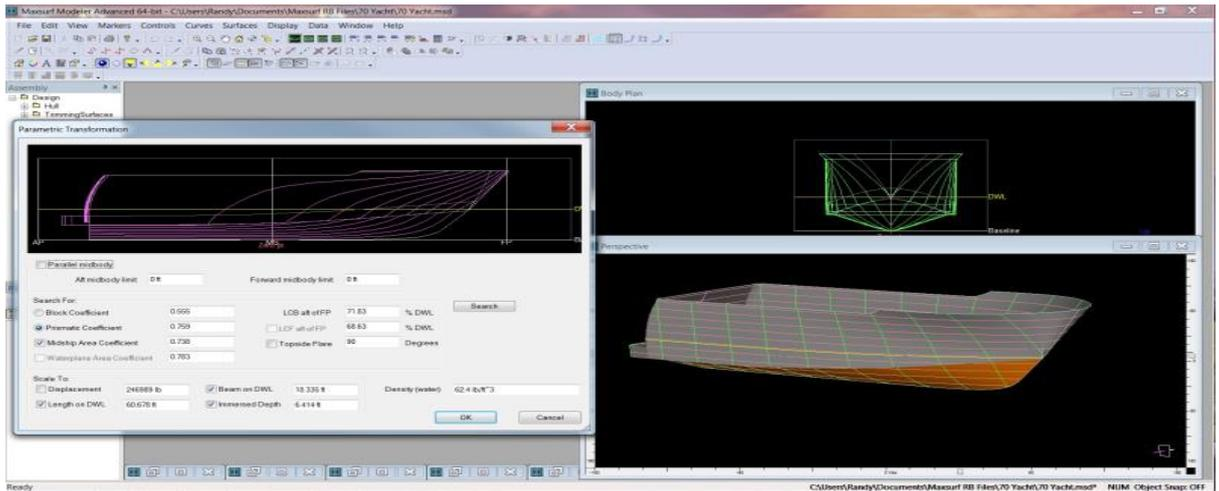
Figure 2: Fishing Boat hull design in maxsurf modeller
