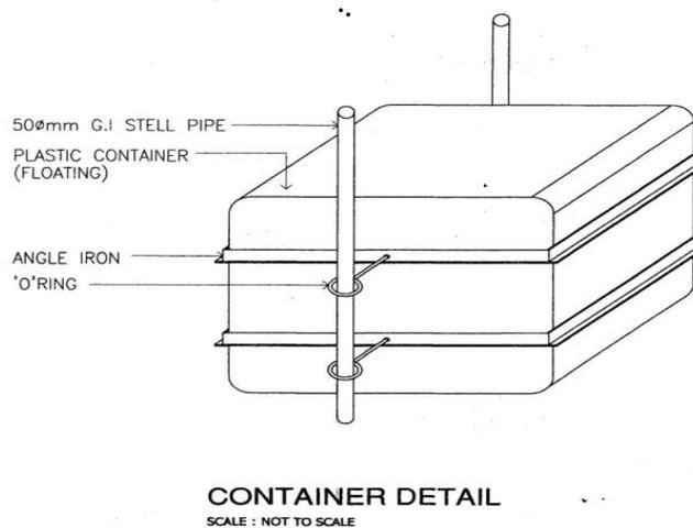
Figure 2: Floating Rubbish Trap Detail
