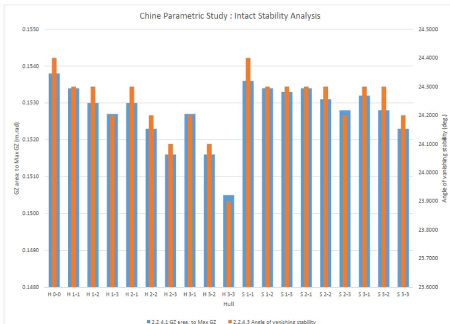
Figure 9: Intact Stability Result
