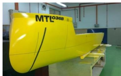
Figure 2: Tanker model with X-bow design, MTL036B
