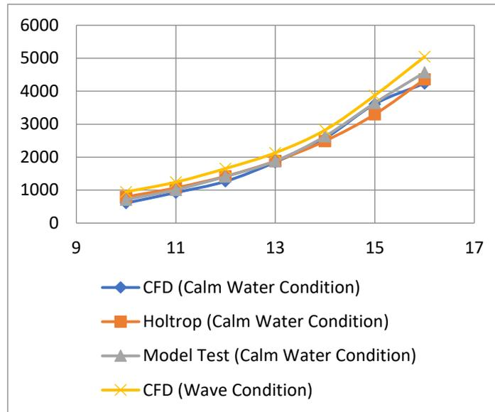
Figure 7: Comparison of total effective power in wave condition using CFD with Holtrop and Model Test in calm water condition
