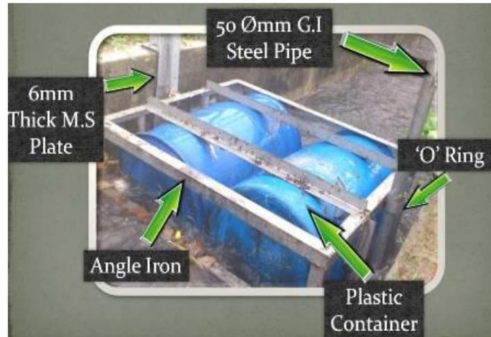
Figure 3: Floating Rubbish Trap Material
