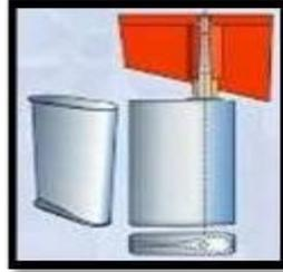
Figure 4: Design Shaped Rudders (Shilling Rudder)
