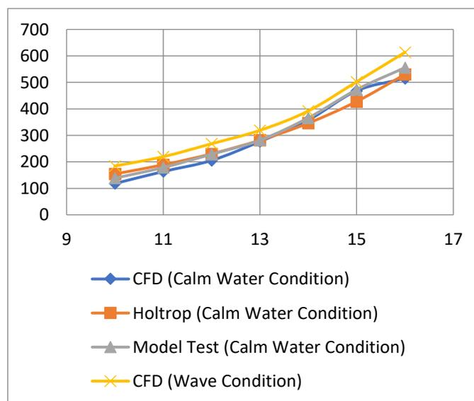
Figure 6: Total resistance versus ship speed graph both in calm water condition and wave condition
