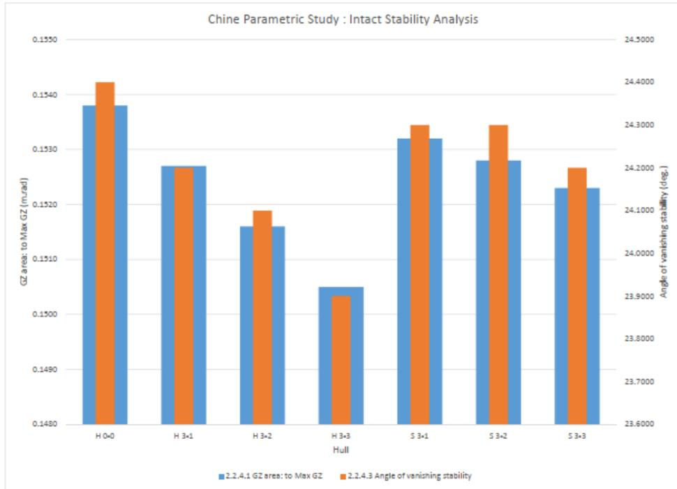
Figure A: Comparison of Chine with Same Chine Width of 3 feet
