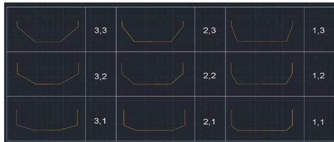
Figure 6: Hard Chine of H 1-1 till H 3-3
